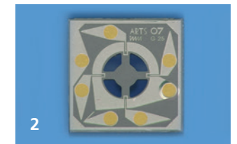
1 Piezo-resistive three-axial force transducer | 2 Sensor backside with piezo resistors and bond pads
