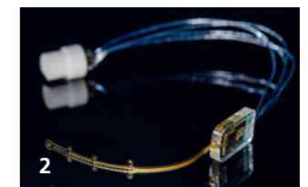
1 Detail of spinal electrode array | 2 Spinal electrode array with interface and electric connector
