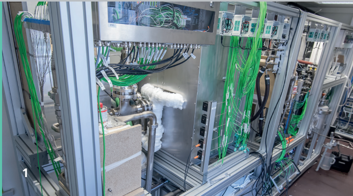
1 Reforming of natural gas / methane / biogas and electricity generation by fuel cell
