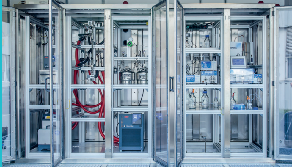
Pilot plant for drug synthesis (in a container)
