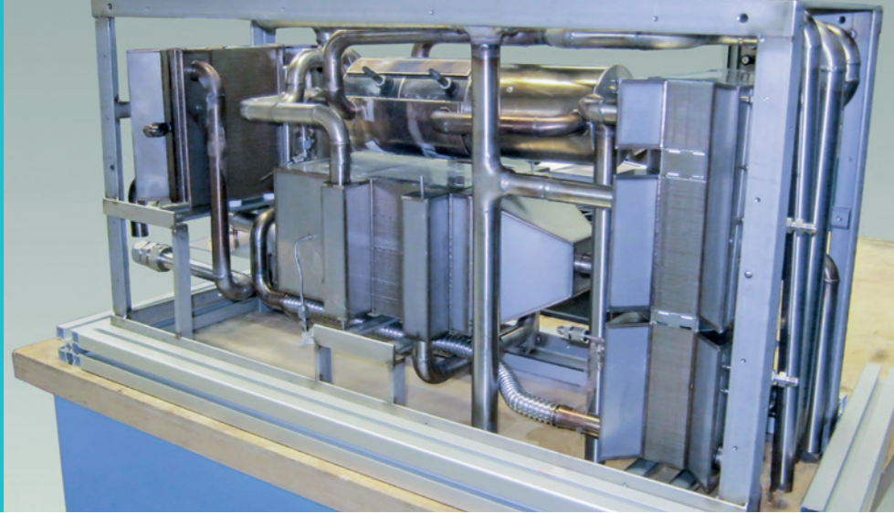
Fuel processor system for the reforming of propylene glycol
