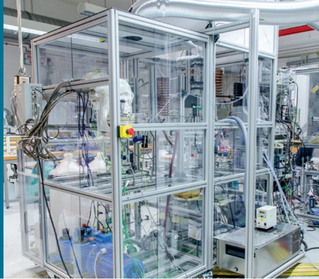
Pilot plant for the production of biodiesel under supercritical conditions
