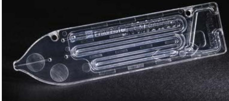
Here, we use the microfluidic device demonstrator CTSelect for automated single cell isolation of circulating tumor cells. A combination of pre-enrichment of the target cells and gentle cell separation in a microchip can enable the isolation of viable tumor cells. In doing so, we aim to generate cross-regional interest in collaboration for personalized therapy discovery in various cancers.
