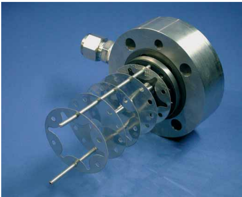
Stacking of the platelets on guiding pins for StarLam3000
