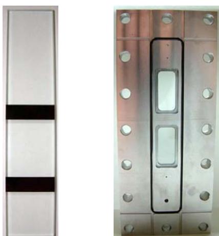
Figure 4: Photography of the cell used for the visualization of the multiphase flow; left – glass channel with embedded glassy carbon electrodes, right – stainless steel framework.
