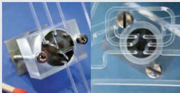
Turning valves integrated on chip
