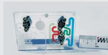
Purification and isolation of mRNA from cervical smears for HPV-detection
