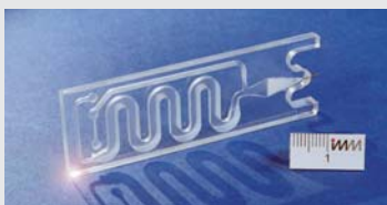
Purification and isolation of DNA from whole blood based on silica beads
