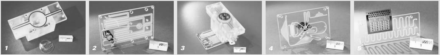
Fig. 2 Incubation module including paddle wheel mixer (1). Separation module with macro-to-micro interface and lysis chamber (2). Integrated unit for cell isolation, enrichment and lysis (3). Amplification module for Reverse Transcriptase MLPA (4) and electrochemical detection module (5).
