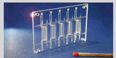
5x parallel transmission and fluores- cence detection cell
