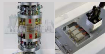
Moving heaters (PCR carousel) for stationary PCR on chip (left) and stationary heating zones (right) for moving plug PCR, for fast nucleic acid amplification
