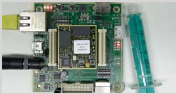
Main board for control logic
