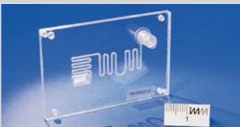
Moving-plug PCR chip for 3 constant temperature zones
