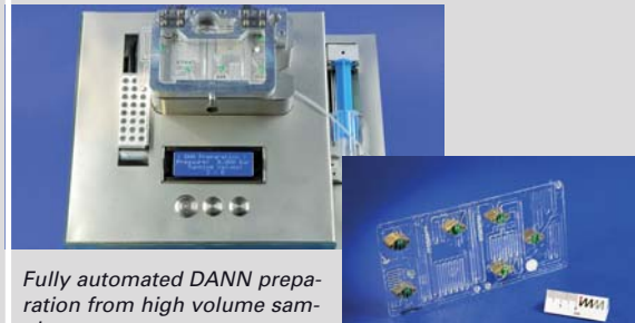
Detection platform for CBRNE (chemical, biological, radiological, nuclear or explosive) substances
