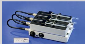
Custom-made freely addressable compact syringe pump
