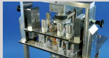
Operating setup harboring all mechanical, electrical and optical components needed to drive the chip automatically
