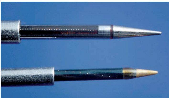
Fig. 2: Detailed view of the linear and helical probe tips
